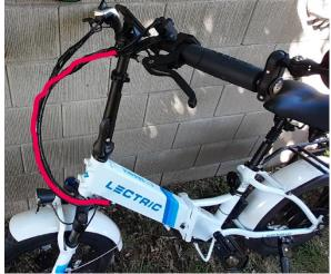
3. Connect the SWITCH PANEL to the SWITCH PANEL CABLE.
