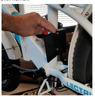
4. **IMPORTANT!** <u>Insert the plastic insulator into the BOX</u>. Now gently re-insert the Circuit Board back into the BOX. Make sure all wires exiting the box are located within the SLOT in the bottom of the BOX and that they do not protrude above the top edge.
