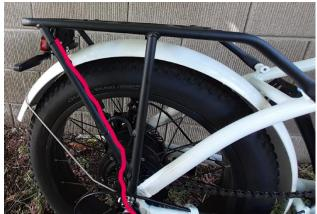
4. Connect the Tail Light connector to the Tail light Cable.
