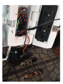
3. Using a **BLUE Scotchlok** Snap Lock connector(supplied), connect the Black wire from the X-1 POWER CABLE to the Black wire on the E-Bike power connector. Do NOT strip this wire.
