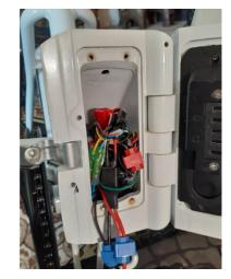
6. In the lower bike cavity carefully locate a two wire, connector that has two wires colored Black and Gray. There are two sets of these. You can use either set. On the side of the connector with the thicker wires, use a **RED Scotchlok** Snap Lock connector (supplied) to connect to the GREEN wire on the X-1 POWER CABLE to the GRAY wire. Do not strip the GREEN wire.
