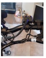
2. Starting at the X-1 CONTROL BOX, connect the SWITCH PANEL cable (5 pin) to the X-1 CONTROL BOX using either end of the cable. Route the cable as shown below, and use tie wraps to secure the cable to the E-Bike at least every 8 inches or so.
