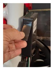
9. Place the last 2" strip of electrical tape over the USB Port. This piece is used as a dust cover for the USB port. Start at the top of the box and completely cover the USB port opening. This piece is placed entirely on the side and is removed when USB charging is used.
